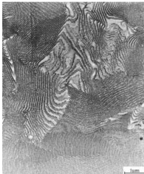
Figure 4. TEM micrograph of SBM40 ( \Phi_{\text{PS}} = 0.40 , M_n = 212 kg/mol) with perforated lamellae of PS (stained with \text{RuO}_4 ).
