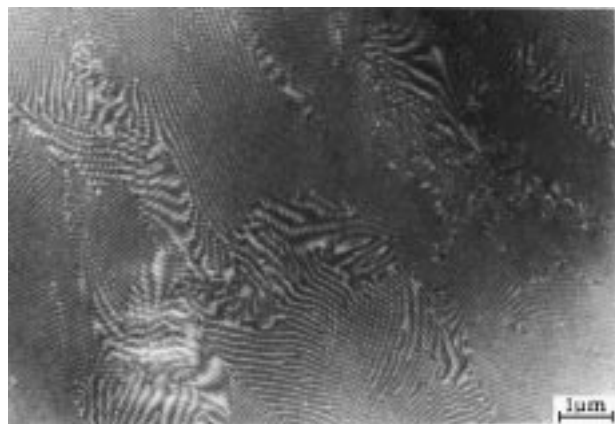
Figure 2. TEM micrograph of SBM76 ( \Phi_{\text{PS}} = 0.76 , M_n = 459 kg/mol) with hexagonally packed PBMA cylinders (stained with \text{RuO}_4 ). The dark annular ring between the gray PS matrix and the light PBMA cylinders correspond to the interface.
