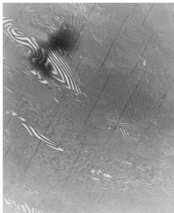
Figure 1. TEM micrograph of SBM72 ( \Phi_{PS} = 0.72 , M_n = 426 kg/mol) with ordered areas of lamellar structures and hexagonally packed PBMA cylinders (stained with RuO 4 ).
